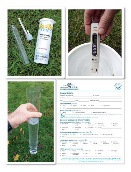
Figure 5. Illustration of the kit and form used by Yealm Dippers when undertaking surveys of water quality as part of the Westcountry Rivers Trust (WRT) Citizen Science Investigation (CSI).
